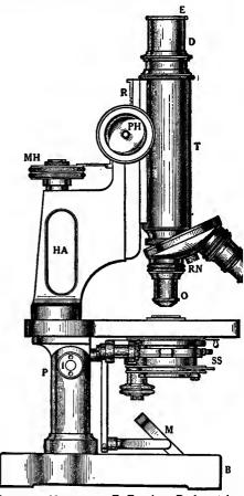
Compound Microscope: E, Eyepiece; D, draw-tube; body-tube; RN, revolving nose-piece; O, objectiv PH, pinion head; MH, micrometer head; HA, hand arm; S, stage; SS, substage; M, mirror; B, base; rack; P, pillar; I, inclination joint.
